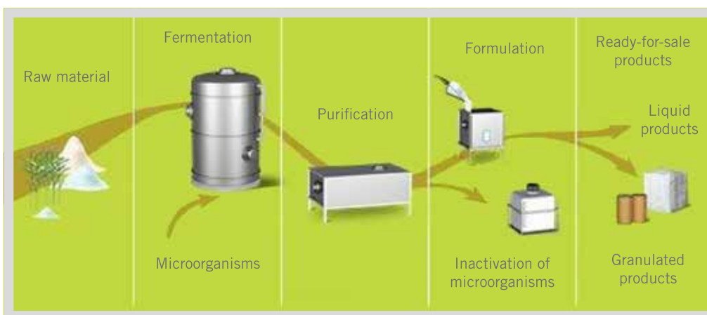
Figure 2 : Main Production Stages for Commercial Enzyme Preparations
